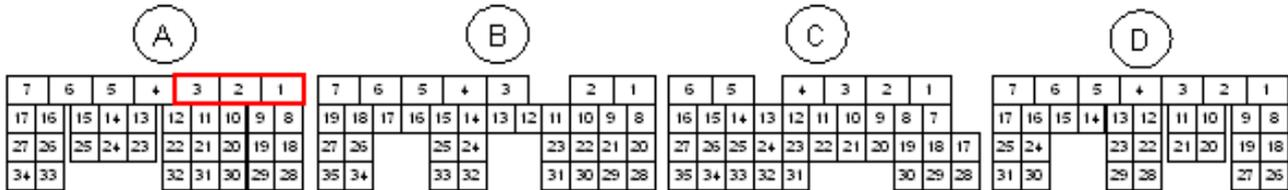
If pins A1, A2 and A3 contain no wires, then the correct ECU required is the *2007 2500cc* version. If these pins contain wires, then the correct ECU is the *2004-2006 2500cc* version.
